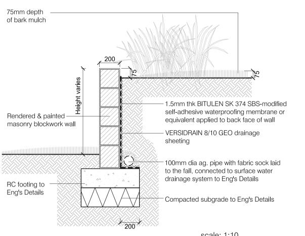
TYPICAL DETAIL 01: retaining wall
